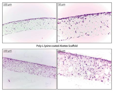
**Figure 1.** Brightfield micrographs showing the structure of 3T3 cells cultured on non-coated and poly-L-lysine coated Alvetex Scaffold discs in 12 well plate format (AVP002) after 7 days culture.
