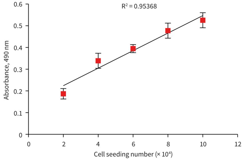
**Figure 3.** MTS standard curve for HepG2 cells (0-100,000 cell number) after 24 hours incubation. 100  $\mu$ L of MTS product removed and absorbance read at 490 nm ( $n = 3$ ,  $\pm$  SEM).
