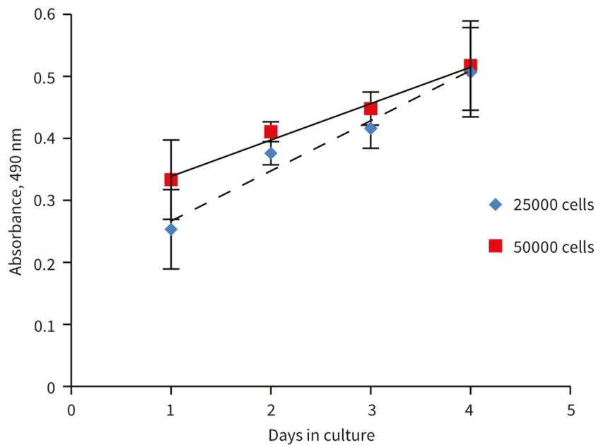
**Figure 4.** MTS growth curves for HepG2 cells grown on Alvetex Scaffold 96 well plate for up to 4 days. HepG2 cells showed good linear cell growth. 100  $\mu$ L of MTS product was removed and read at 490 nm ( $n = 3$ ,  $\pm$  SD). Linear HepG2 growth was observed for up to 4 days at both 25,000 and 50,000 cells per well seeding density ( $R^2 = 0.963$  and  $0.985$  respectively).
