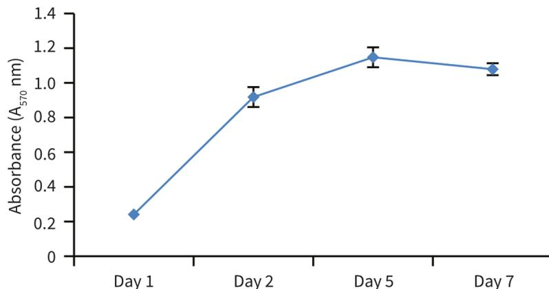
**Figure 8.** Cell viability growth curve (MTT assay). HepG2 cells were seeded at a density of 100,000 cells per well onto Alvetex Scaffold 96 well plate format and subsequently monitored over a 7 day period. Cell growth proceeded through an initial log phase and then reached a plateau by day 5, after which time the viability began to decline;  $n = 3, \pm \text{SEM}$ .
