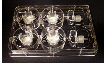
Example: Alvetex Perfusion Plate showing 4 × Alvetex 12 Well Inserts in position
