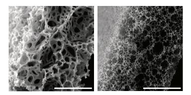
Scanning electron micrographs of Alvetex Scaffold (left) and Alvetex Strata (right) in transverse section. Scale bars: 100 μm.
