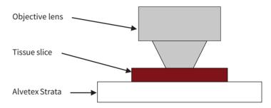
**Figure 2.** Experimental set-up showing maintenance of tissue slice on Alvetex Strata and positioning of objective microscope lens.
