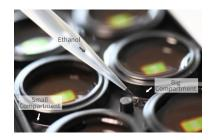
Figure 3: Filling Compartments between Wells with 70% Ethanol
