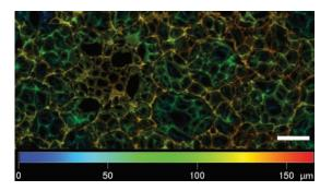
**Figure 9:** Depth colour-coded Z stack of cell-free Alvetex Scaffold stained with Nile Red. Picture taken on a Zeiss LSM 510 confocal microscope. Note the depth of the Z-stack exceeds 150  $\mu$ m. Scale bar 50  $\mu$ m.
