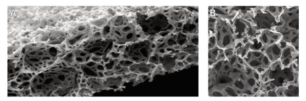
Scanning electron microscope image of Alvetex Scaffold, to highlight its porous structure. **A**: a 200  $\mu$ m thick Alvetex Scaffold disc. **B**: Close up of Alvetex Scaffold voids with dimensions of approximately 42  $\mu$ m in diameter and interconnects of approximately 13  $\mu$ m in diameter.
