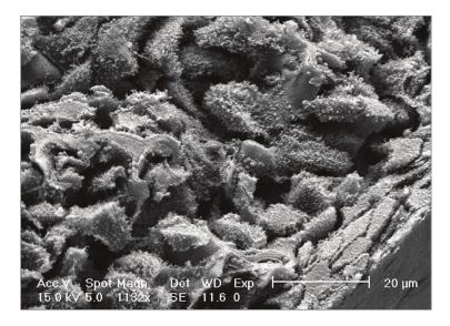
Visualization of the structure of 3D cultures in Alvetex Scaffold is made possible using scanning electron microscopy (SEM). Samples are prepared in the same manner as would normally be used for tissues. In this example, skin, cells have penetrated throughout the scaffold and some have stratified on the surface (lower right corner).
