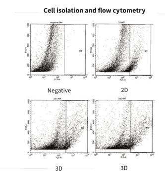
It is possible to isolate some viable cells from Alvetex for downstream experiments such as flow cytometry, cytospinning and for subculture. Here, mesenchymal stem cells induced to form adipocytes were isolated from Alvetex Scaffold and 2D cultures. Cells were subsequently stained with Nile Red to detect the presence of lipid and analyzed by flow cytometry.
