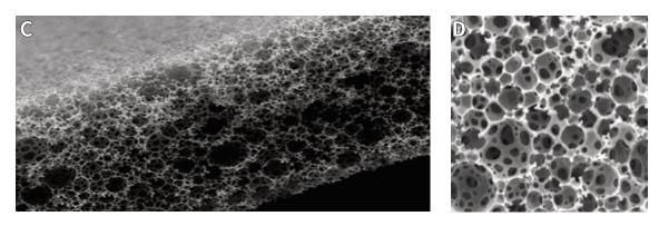
Scanning electron microscope image of Alvetex Strata. **C**: a 200  $\mu$ m thick Alvetex Strata disc. **D**: Close up of Alvetex Strata voids with dimensions of approximately 15  $\mu$ m in diameter and interconnects of approximately 5  $\mu$ m in diameter.
